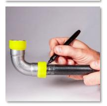
5. Ensure that press fitting components are intact and seated properly. Refer to illustration for proper fit of grip ring, separation ring, and sealing element.
