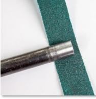
3. Remove all burrs from the inside and outside of pipe and prepare pipe surface to insertion depth using deburring tool or fine grit sandpaper.
