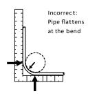
NOTE: Tubing may be bent to a minimum of 5 x O.D. with approved bend support.
