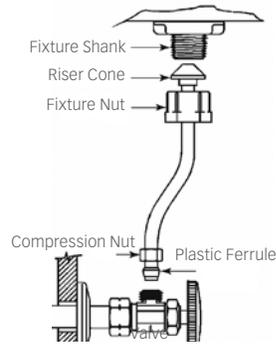
Slide compression nut and supplied plastic ferrule over tube as shown. The long taper of the ferrule goes towards valve. Thread fixture nut onto valve. Tighten fixture nut hand tight plus an additional 1/2 turn.
