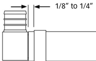
3. Insert the fitting into the pipe to the shoulder or tube stop. Position the ring 1/8" to 1/4" from the end of the tubing.
