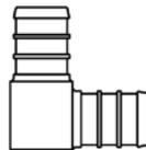
For bends smaller than 8 x outside tube diameter, install an elbow fitting
