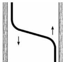
In the normal process of installing tubing, slack is generally provided by snaking the tubing around obstacles and by some sagging between supports. A change in direction offset or loop can be used when slack requirements are not met by these other installation methods.
