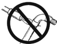
**NOTE:** Never expose CANPEX to direct flame or high temperatures. Proper installation procedures can help ensure the long life of the CANPEX plumbing system. Braze, solder or weld any metallic fittings and allow to cool **BEFORE** you connect them to CANPEX.
