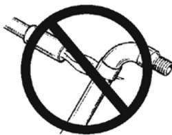
PEX tubing systems should not be intentionally subjected to freezing. Do not use open torch or excessive heat to thaw PEX tubing. Tubing failure or damage can result. Heat must be applied directly to the frozen tubing section. Temperature on tubing shall not exceed 180°F.
