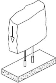
Protect the CANPEX tubing with non-metallic sleeving material where it **enters and/or exits a concrete slab**. CANPEX need not be sleeved its entire length within the slab. However, full length sleeving is allowed.
