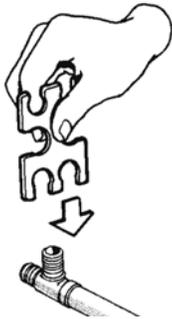
2. Slide the correct size "GO" side of the crimp gauge over the crimp ring at least FOUR places. **DO NOT** gauge the crimp at the jaw overlap area.
