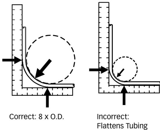
**DO NOT bend CANPEX** in a radius smaller than eight (8) times the outside diameter of the tubing. Flattened tubing is damaged and must be cut out and replaced.
