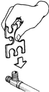
5. When checking crimps with a GO/NO GO gauge, push the gauge STRAIGHT DOWN over the crimped ring. NEVER slide the gauge in from the side. Do not attempt to gauge the crimp at the jaw overlap area.
