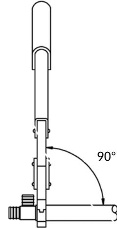
4. The ring must be attached straight. Center the crimping tool jaws exactly over the ring. Keep the tool at 90° and close the handles completely. **DO NOT CRIMP TWICE.**
