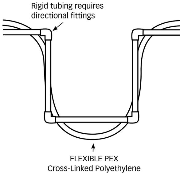
CANPEX tubing is flexible, reducing the need for most directional fittings
