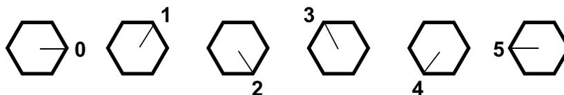
To reduce crimp size, rotate Back Pin to next higher number
