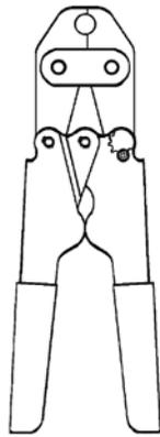
2. Note the position of the notched head of the adjustment cam in relation to the Phillips-head retaining screw.
