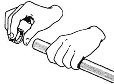
2. Slide the correct size blackened copper crimp ring over the tubing end.
