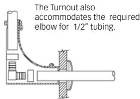
The connection of CANPEX distribution lines to individual fixtures may be accomplished with a variety of fittings available from Vanguard. CANPEX may be stubbed directly out of the wall with the use of a Turnout. At floor levels above a crawl space, basement, or on upper floors, it may be desirable to run the tubing through the floor directly to the fixture, rather than behind the wall.
