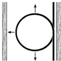
CANPEX expands or contracts 1" in every 100' of pipe for every 10°F of temperature change. You should allow for this expansion and contraction in your installation procedures. **ALWAYS** cut the pipe too long.
