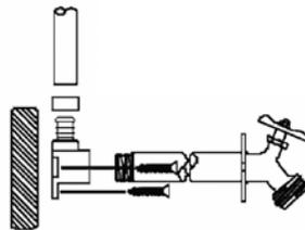
Free Standing Hose Bibbs shall not be supported by CANPEX. Well anchored drop ear fittings or metal pipe shall be used to install hose bibbs.
