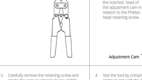
rotate the cam counterclockwise slightly until the retaining screw can be installed in the other threaded hole. This provides about 1/2 notch of adjustment.
