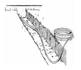
Snake tubing from side to side to allow for tube contraction.
