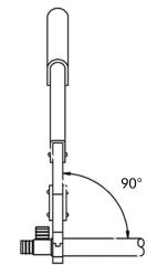
4. The ring must be attached straight. Center the crimping tool jaws exactly over the ring. Keep the tool at 90° and close the handles completely. **DO NOT CRIMP TWICE.**
