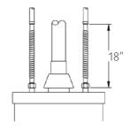
Use metallic connectors to attach CANPEX to **GAS WATER HEATERS.** Install a minimum 18" of metallic or other piping between the water heater and CANPEX.
