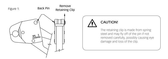
From the clip end of the back pin, push it towards the tool body until the hex head on the other end of the pin just clears the body.
