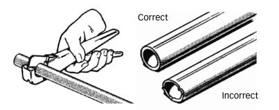
1. The tubing should be cut squarely and evenly without burrs. Uneven, jagged or irregular cuts will produce unsatisfactory connections.
